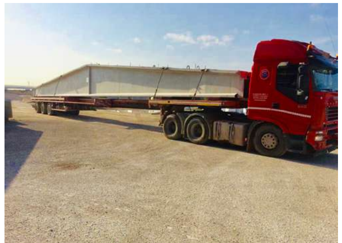
» Double-slope beam transport DELTA system
